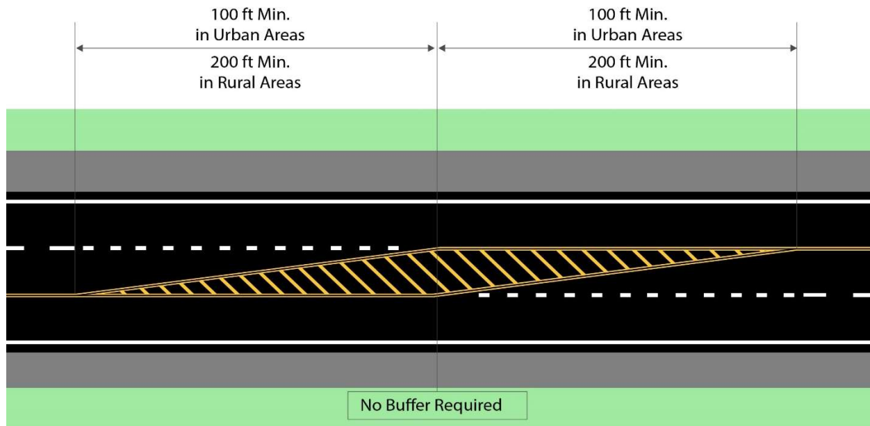
Figure 3 Schematic for Tail-to-Tail Transitions on a 2+1 Roadway
